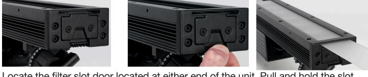
Locate the filter slot door located at either end of the unit. Pull and hold the slot door down and gently slide the frost/diffuser filter in. Make sure the filter is all the way inside before releasing the slot door to close.
